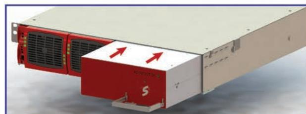
Using Handle, gently push By-Pass Module into the shelf
